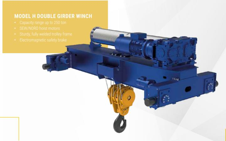
The **EMH Model HF double girder winch** is a winch made for the large capacity range. The parallel shaft gearbox braking motor connected at the face end offers a favourable alternative to a large winch because the basic structure can be derived from the standard series. The open design of the winch ensures ease of maintenance and servicing.
