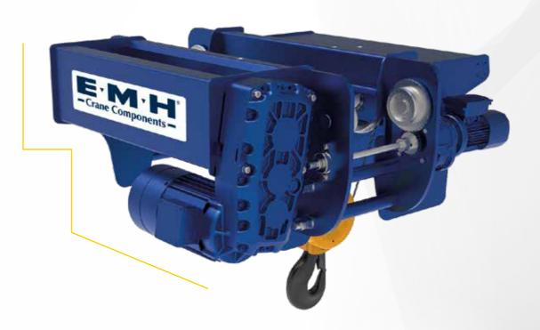
The **EMH Model E single girder hoist** is notable for its highly favourable approach and hook dimensions. These are achieved with a compact, fully welded frame adapted to provide the best match for all the components used. The parallel configuration of the rope drum and the hoist motor also contribute to the overall compact size of the Model E short trolley. In addition, this configuration ensures easy servicing and maintenance.
