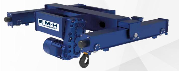
The **EMH Model DL double girder hoist** is a compact wire rope hoist for the medium capacity range. Due to the lowered design of the height, this model is the optimal solution for low room heights and lack of space above the crane main girder. A one-sided articulated running gear carrier connection ensures that all trolley wheels make full contact. In this way, the forces resulting from crane use are optimally distributed to the substructure.
