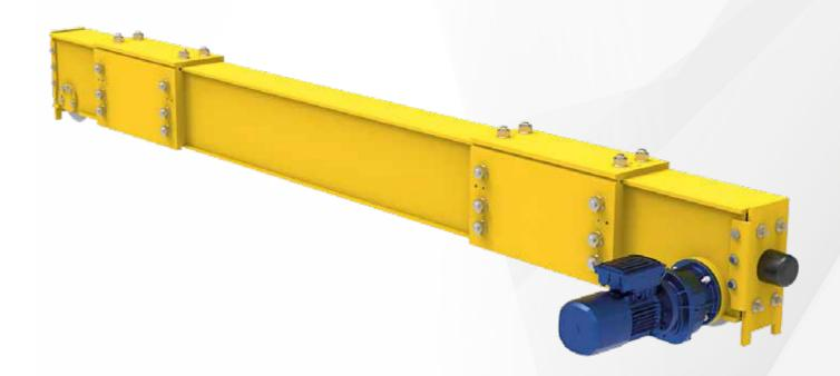
The **EMH Model HSZ endtruck for double girder overhead cranes** is our endtruck for double girder overhead cranes. The sturdy, fully welded frame, completely machined in one set-up, complies with the strictest quality standards. The surface-hardened wheels are turned from solid and run extremely smoothly because of the roller bearings and the precision manufacturing.
